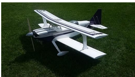
1/4-scale Ultimate Bipe with DLE 55 engine.
